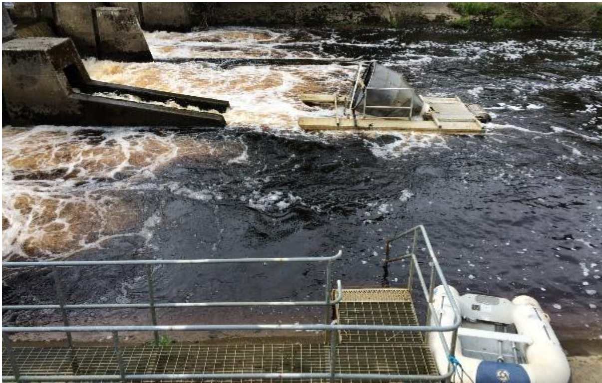
Fig 2. RST in the non-fishing position with the drum raised. Note access gangway and boat used to access the RST.
